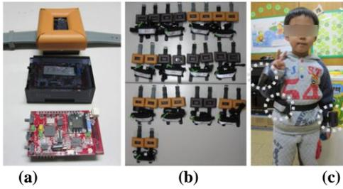
**Figure 1. (a) The sensor (b) The entire stock of sensors (c) A child wearing three sensors**
